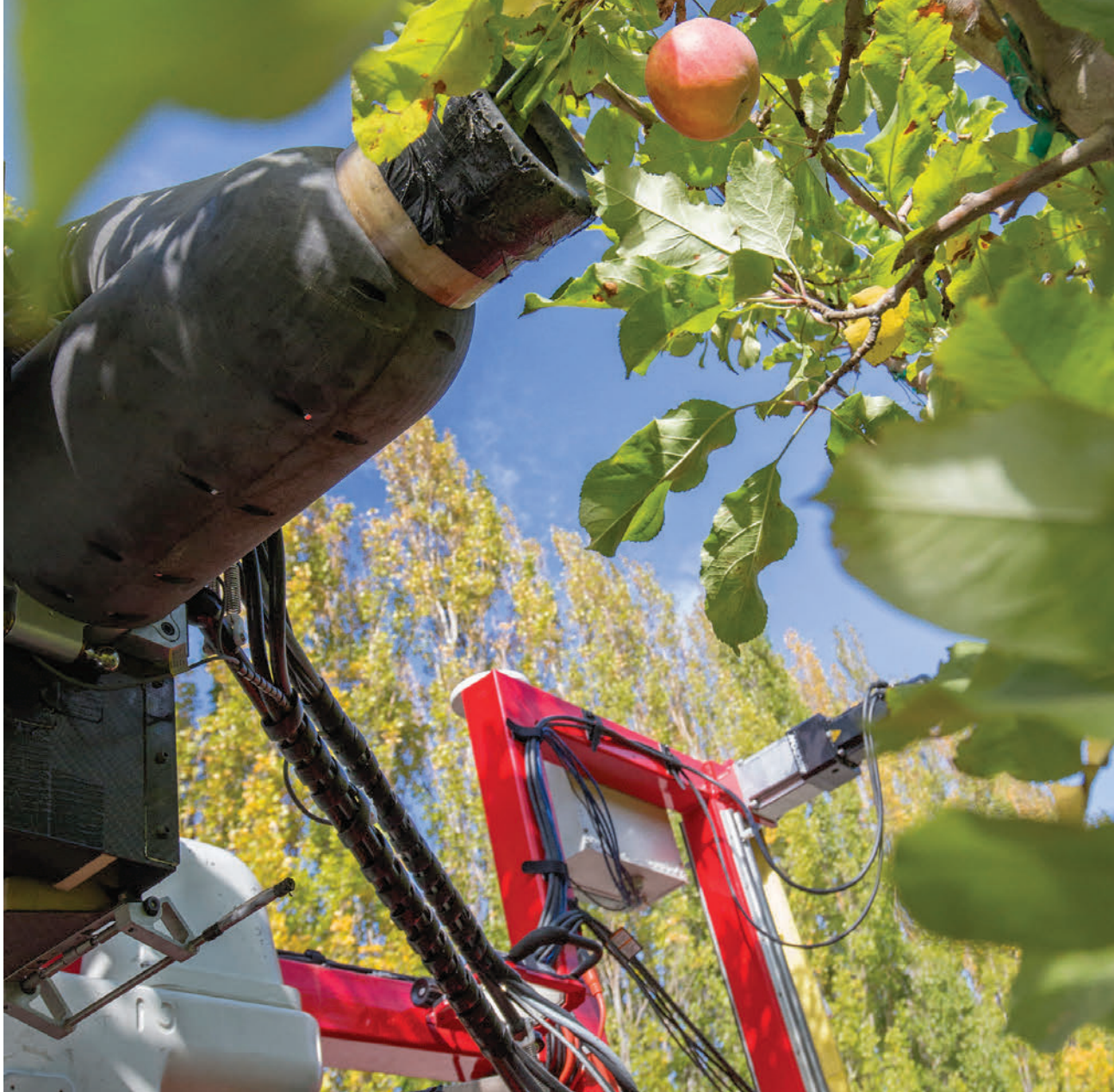
A Fuji apple is sucked from a tree during the 2016 Washington apple harvest during a demonstration of an automated vacuum harvester by Abundant Robotics.
