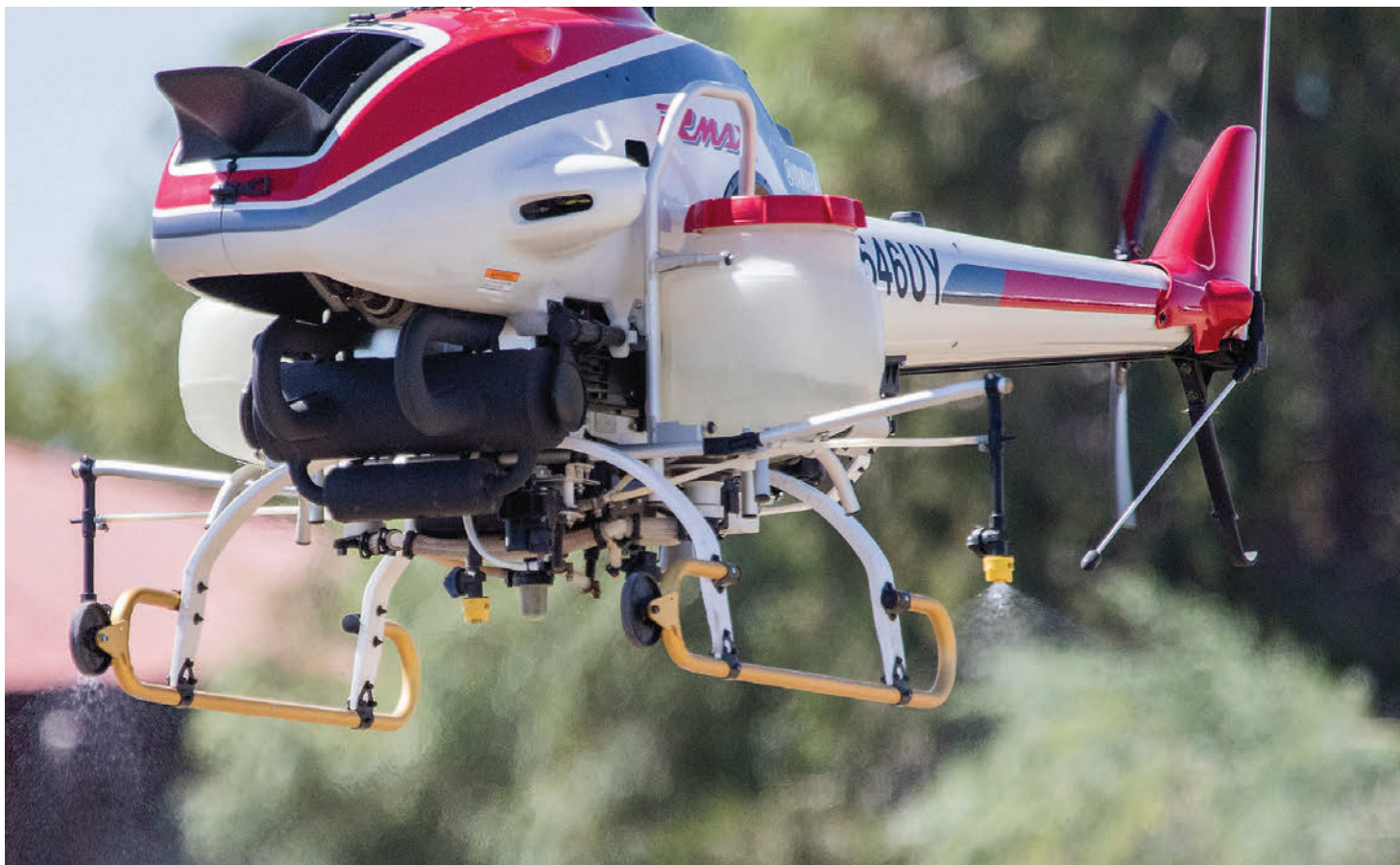
A Yamaha RMax UAV flies a prearranged flight path to spray from two tanks filled with water over a field. The capacity of each tank is about 2 gallons.
