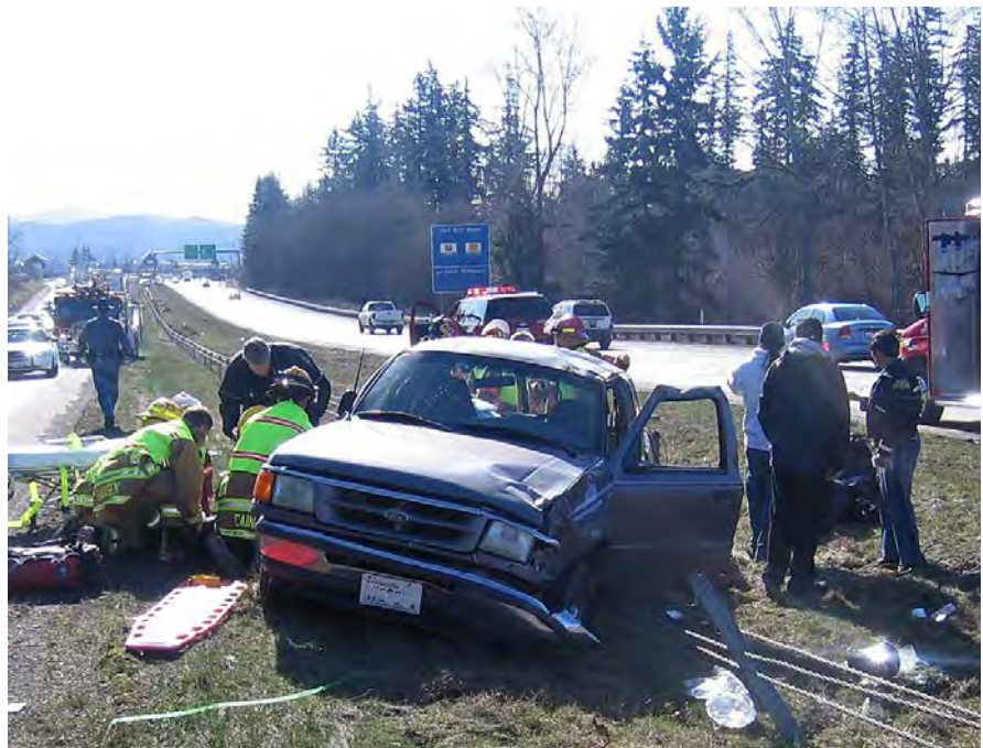
Three-strand cable barrier on I-5 near Bellingham prevented this vehicle from crossing over the highway median into oncoming traffic.
