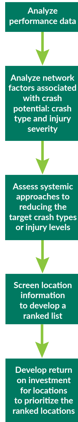
Exhibit 13. I-2 Safety Program General Process Flow
